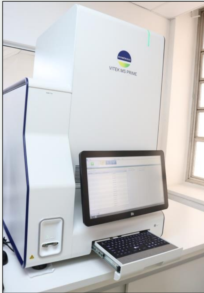
Equipamento MALDI-TOF ( Matrix Assisted Laser Desorption Ionization Time Of Flight)
